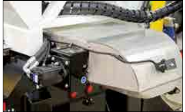
Fig 58 - Slave conveyor drive
