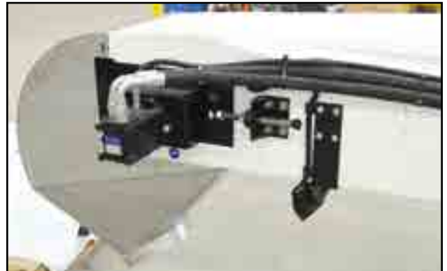
Fig 59 - Rear conveyor drive
