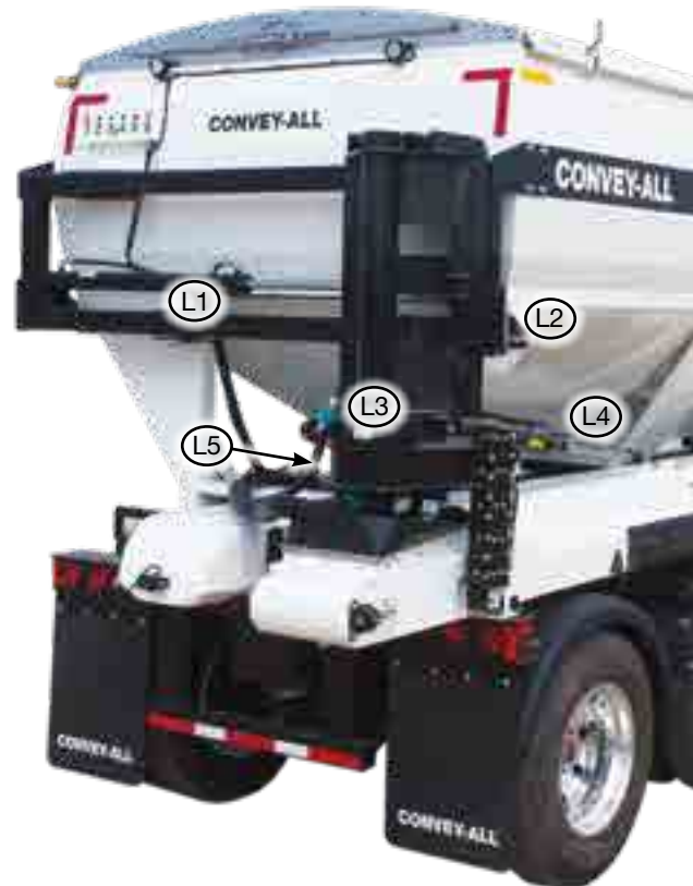
Fig 19 - Limit switches controlling rear conveyor movements
