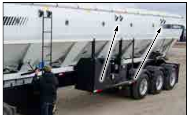
Fig 32 - Exterior ladder brackets
