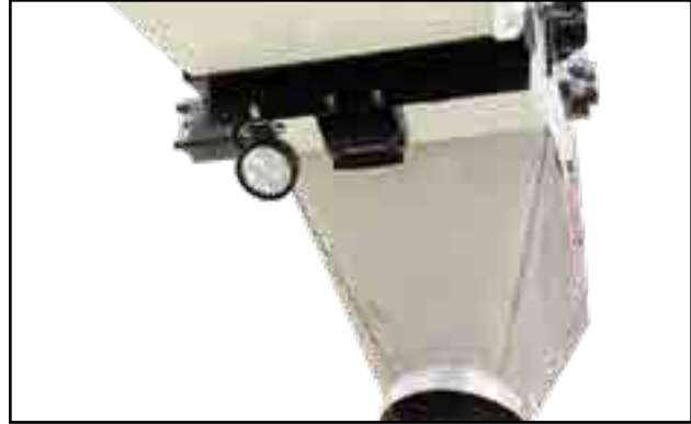
Fig 26 - Light and camera on rear conveyor discharge
