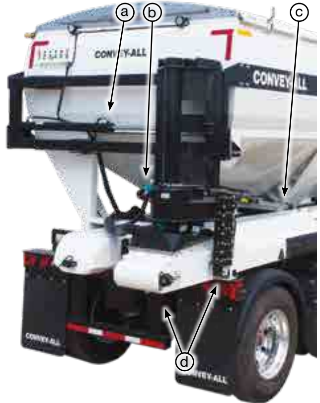
Fig 62 - Rear conveyor movement points
