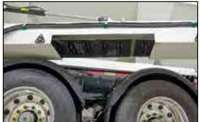
Fig 70 - Rear conveyor, access panel removed
