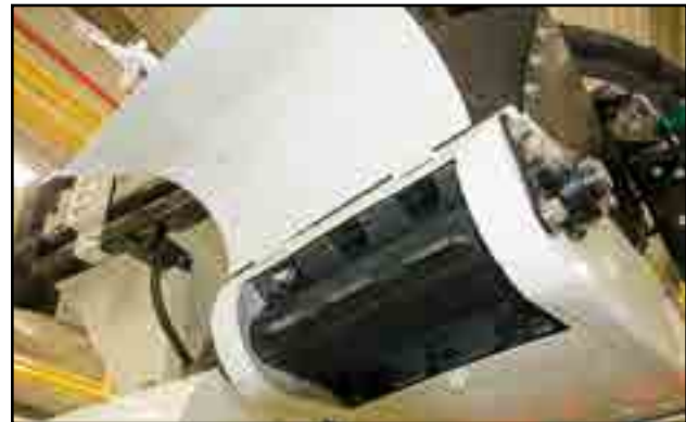
Fig 20 - Hopper access panel
