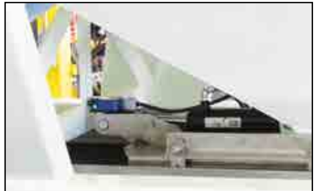
Fig 48 - Compartment gate cylinder
